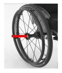
The axle is not secure until the outside quick-release button pops out to its fully extended position (the ball bearings on the opposite end of the axle must be fully visible beyond the end of the axle sleeve). Check to make sure the axles are locked; excessive play should not exceed 2 mm.
