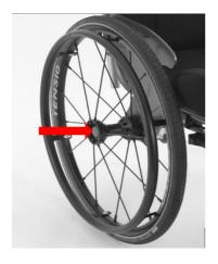
The axle is not secure until the outside quick-release button pops out to its fully extended position (the ball bearings on the opposite end of the axle must be fully visible beyond the end of the axle sleeve). Check to make sure the axles are locked; excessive play should not exceed 2 mm.
